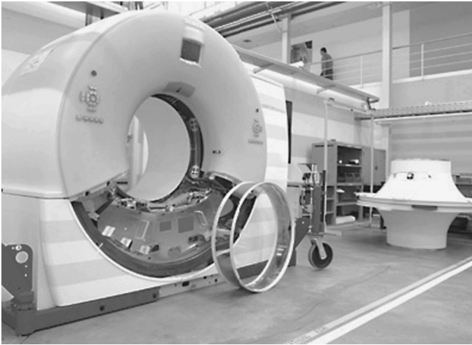
Fig. 1.12. Manufacturing of a modern CT scanner. (From Siemens web site.)
